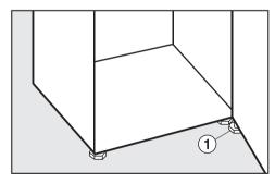
Also unscrew support ① from the bearing block, to level the appliance door.
